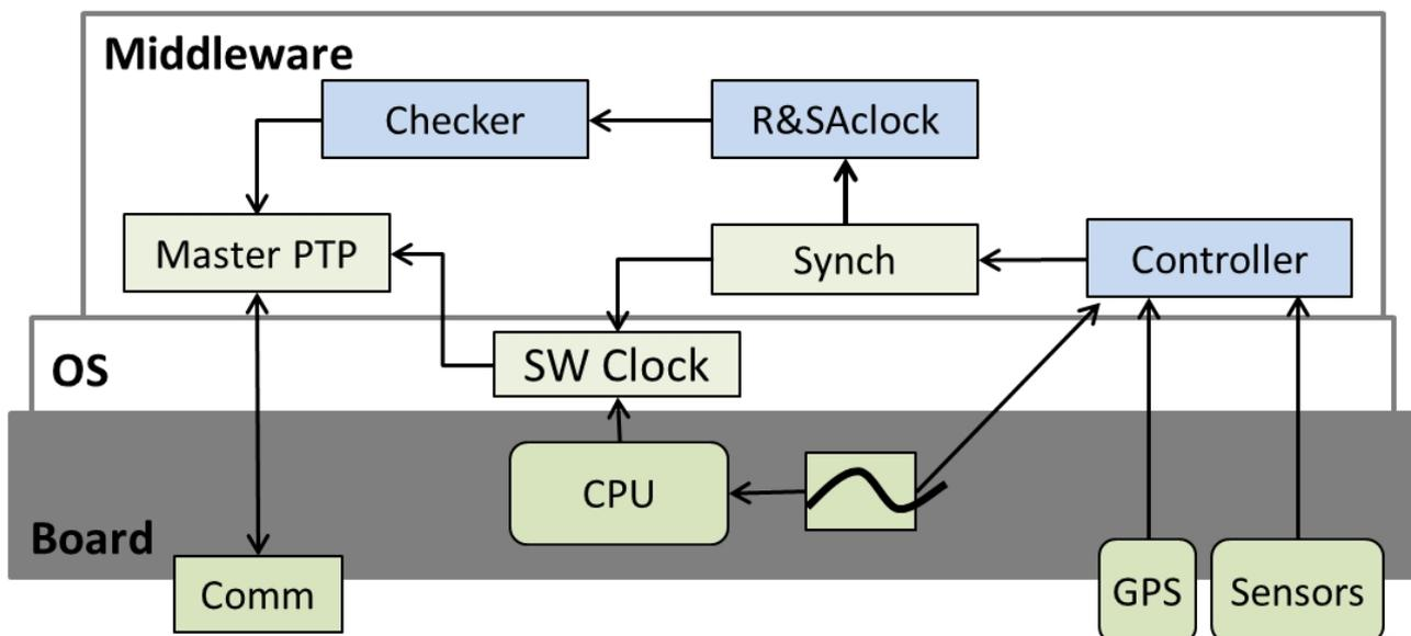
Figure 1 : The Resilient Master Clock architecture
